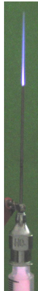
Fig. 2. Photograph of the plasma plume. Applied voltage: 8 kV; pulse frequency: 10 kHz; pulsewidth 500 ns; working gas: He/ \text{O}_2 (20%); and total flow rate: 0.4 L/min.
