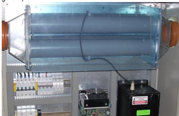
Figure 2: View of the modular low-temperature plasma generator with mesh electrodes
