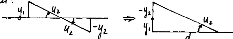
$$\begin{aligned} \tan u_2 &= \frac{y_1 - y_2}{d} \Rightarrow d \cdot u_2 = y_1 - y_2 \Rightarrow y_2 = y_1 - d \cdot u_2 = \\ &= y_1 - \frac{d}{n_2} \cdot \underbrace{u_2 \cdot n_2}_{= V_2} \stackrel{(1)}{\Leftrightarrow} y_1 - \frac{d}{n_2} \left( \frac{n_2 - n_1}{R_1} \cdot y_1 + V_1 \right) \Rightarrow \end{aligned}$$
